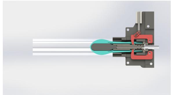
*Figure 3 Torpedo launching mechanism*
