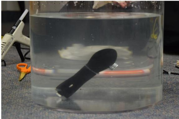
*Figure 5 Torpedo buoyancy tests*
