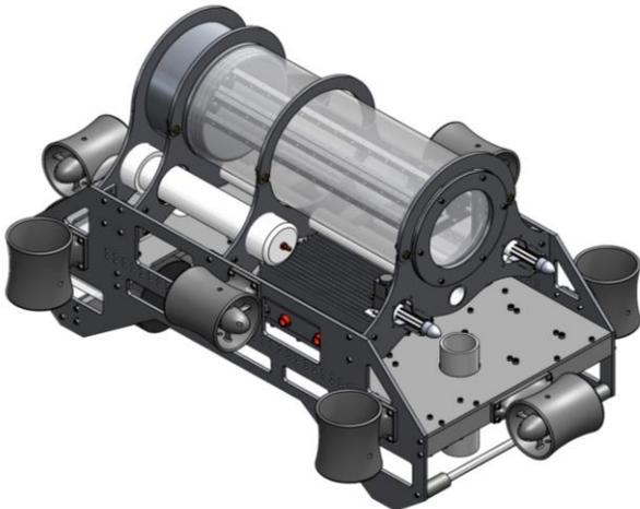
Figure 2: Polaris, AUVIC's Current AUV
