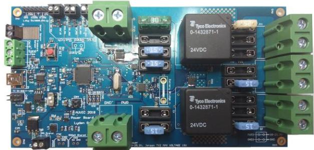
Figure 3: Power Regulation Board (Top Layer)
