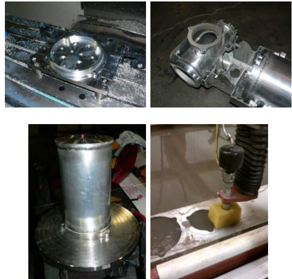
Figure 3: Top Left: CNC machining of an endcap, Top Right: DVL box in the main frame, Bottom Left: Welding of a battery pod, Bottom Right: Waterjet cutting.
