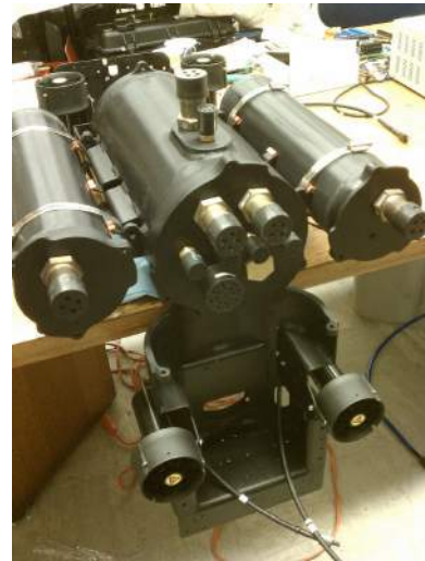
Figure 2: Demonstration of folding weldments which allow access to bulkheads and internal computer pressure vessel components through endcap removal.
