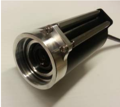
Figure 11: Camera pressure vessel assembled with uEye camera.
