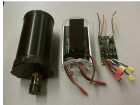
Figure 10: Battery pod pressure vessel and internal configuration.
