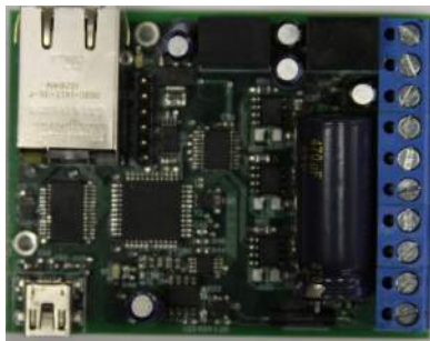
Figure 6: Motor control hardware.
