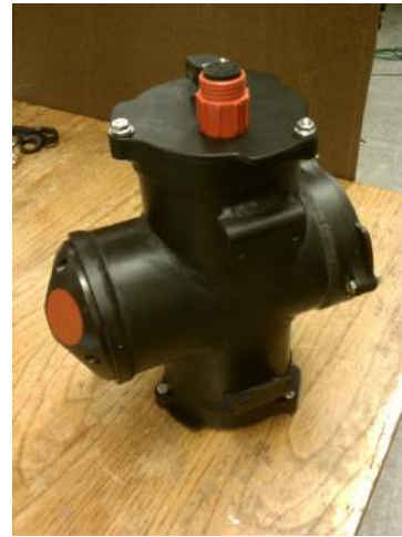
Figure 9: Navigation pressure vessel.
