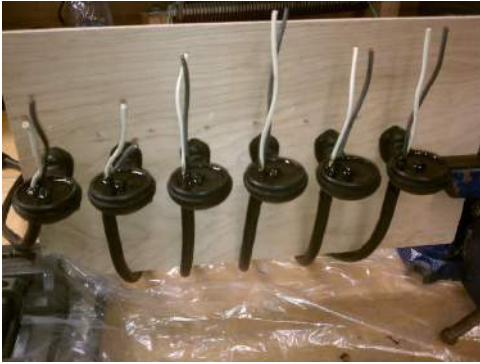
Figure 4: Custom cable potting for thrusters.
