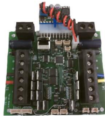
Figure 7: Power management and merge hardware.
