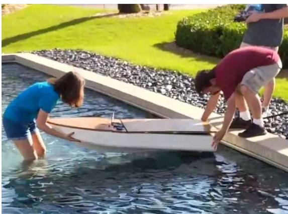
Figure 5: The Double Precision ASV being lowered into the water for a test of remote control operation.
