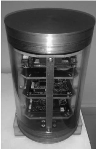
Fig 5. On board electronics inside housing.
