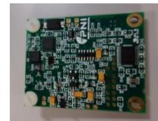
Fig. 15 Attitude sensor (PNI Sensor Corporation: TRAX)
