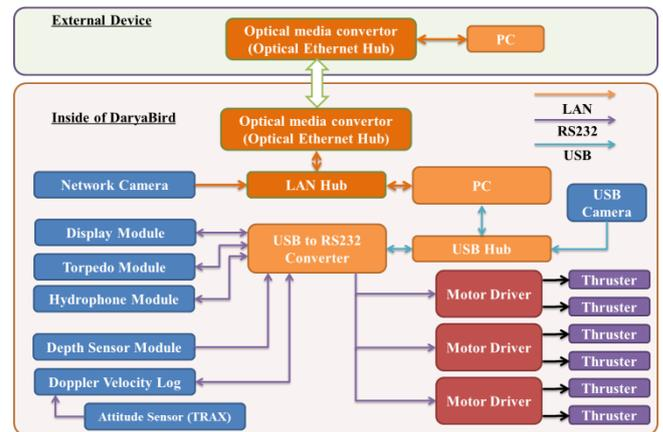
Fig.3 System architecture of DaryaBird
