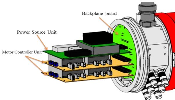
Fig.7 Motor Controller Unit
