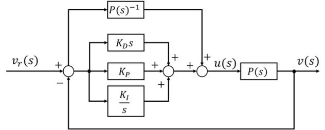
Fig.19 Velocity Control system (Surge&Sway)
