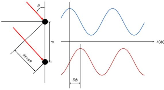
Fig.16 Sound source localization based on SSBL
