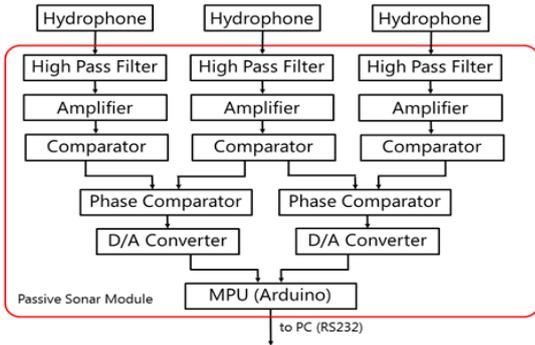
Fig.17 Passive Sonar System
