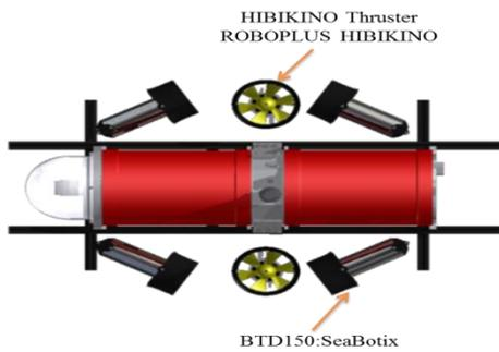
Fig.6 Arrangement of thrusters
