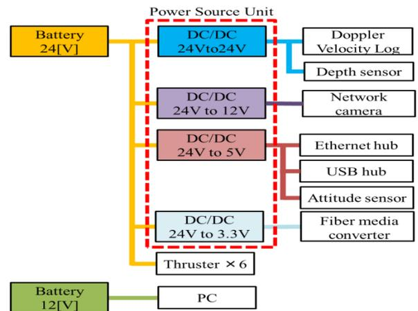
Fig.8 Power supply system
