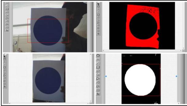
Figure 10: Recognizing a Blue Circle using Vision Processing
