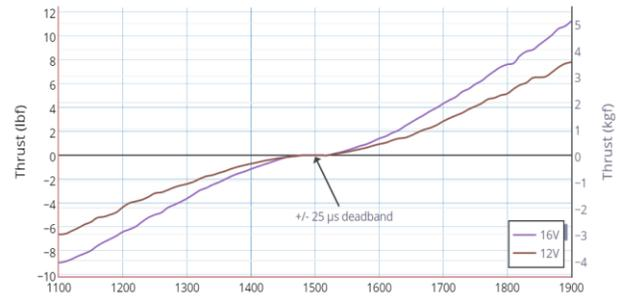
Figure 5: Thrust vs. PWM input [2]
